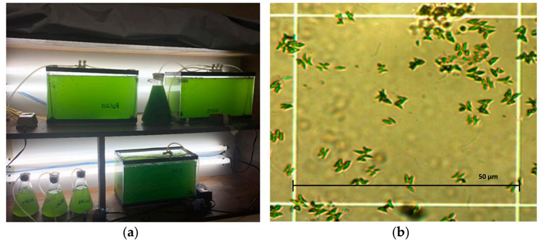
**Figure 1.** (a) Inocula and containers for the growth of the algae *Scenedesmus* sp. (b) Photomicrograph of *Scenedesmus* sp. grown in an aquarium during the study, as visualised under optical microscopy at 100× magnification.
