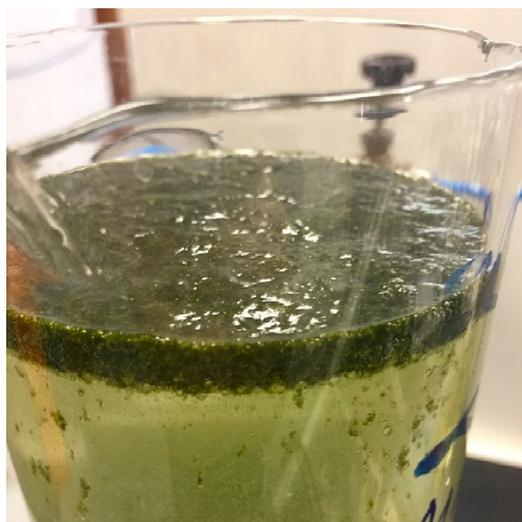
**Figure 7.** Floated biomass in the coagulation-DAF experiments for microalgae removal. Conditions: 0.3 mL L<sup>-1</sup> Tanfloc SG; 2 mg L<sup>-1</sup> anionic polyacrylamide; pH = 8 ± 0.1; a saturation pressure of 5 atm; and a recycle ratio of 20%.
