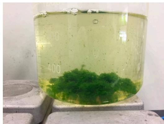
**Figure 6.** Settled flocs of microalgae after coagulation and flocculation. Conditions applied: a pH of 8.0+/-0.1; 0.3 mL L<sup>-1</sup> of Tanfloc SG; and 2 mg L<sup>-1</sup> of flocculant (Floerger AN 956 SH).
