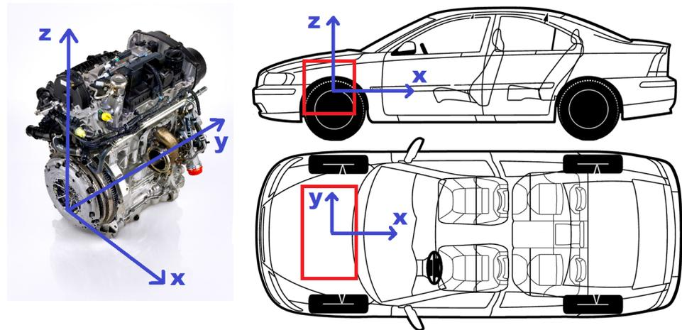
**Figure 1.** Powertrain and vehicle coordinate systems. The red rectangle represents the powertrain's position within the vehicle.
