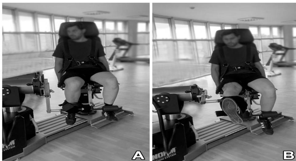
**Figure 3.** The knee flexion (A) and extension (B) movements by the isokinetic dynamometer.
