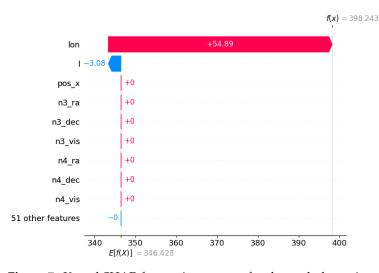
**Figure 7.** Kernel SHAP feature importance for the peak datapoint. The spacecraft geographical longitude is the most critical feature in determining the sudden count rate increase from a baseline count rate of 346 to 398 (the peak). This baseline is constructed using 15 datapoints before and after the peak, which are used for sampling values and perturbing the datapoint to provide an explanation.
