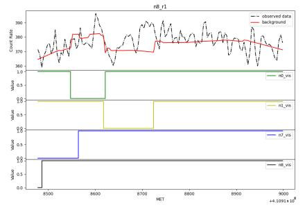
**Figure 8.** Observed and estimated count rate light curve for detector n8 in energy range *r*1. The unexpected steps in estimated count rates are attributed to variations in features such as n0\_vis, n1\_vis and n7\_vis, with n8\_vis remaining constant during this unusual estimation period.
