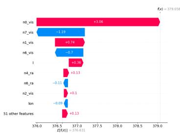
**Figure 9.** Kernel SHAP feature importance for a datapoint in a step of the estimated background in Figure 8. Notably, the most influential features are those related to detector visibility, specifically whether the FoV is obscured by the Earth or not. The baseline for this method is established by using 15 datapoints before and after the datapoint to be explained. These datapoints are used for value sampling and perturbation of the datapoint during the explanation process.
