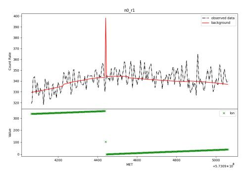
**Figure 6.** Light curve of observed and estimated count rates for detector n0 in energy range r1. An unexpected peak appears in the estimated count rates due to an error in the dataset for the longitude estimation.
