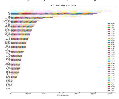
**Figure 4.** Feature importance as determined by the Morris method for the 2019 dataset. Features are ranked by average importance, with the McIlwain L-parameter and Fermi longitude coordinate at the top. Conversely, certain detector flags indicating the Earth's FoV occultation emerge as almost irrelevant factors in prediction. For a complete list of features and their descriptions, refer to Tables 2 and 3.
