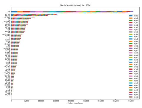
**Figure 5.** Feature importance as determined by the Morris method for the 2014 dataset. Features are sorted by their average importance, with the McIlwain L-parameter and Fermi longitude coordinate as the most influential. In contrast to Figure 4, detector flags representing the Earth's FoV occultation play a significant role in prediction. For a complete list of features and their descriptions, refer to Tables 2 and 3.
