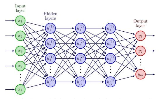
**Figure 1.** The architecture of a feed forward neural network. The input has a dimension of 60. The first two hidden layers have 2048 neurons, the third 1024. The output layer has a dimension of 36.
