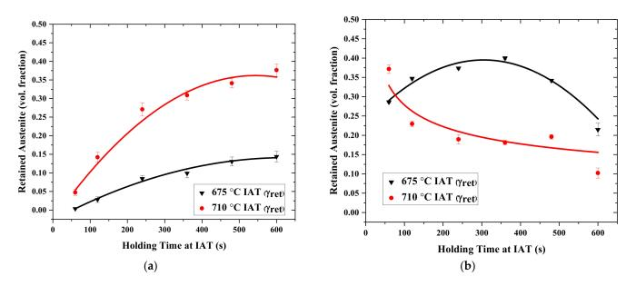
**Figure 5.** Retained austenite volume fraction as a function of intercritical annealing temperature and holding time for (**a**) CR and (**b**) M starting microstructures.
