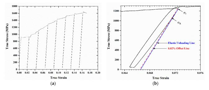
**Figure 2.** (a) Load–unload–reload test; (b) enlarged portion of (a) showing process for determining  $\sigma_F$  and  $\sigma_R$ .
