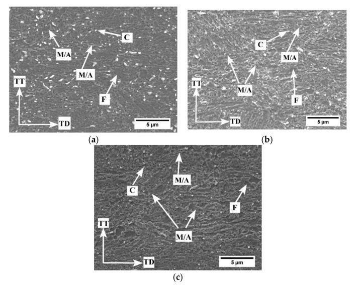
**Figure 7.** SEM micrographs of CR samples annealed at 710 °C for (**a**) 120 s, (**b**) 240 s, and (**c**) 600 s; C = carbide, F = ferrite, M = martensite, and A = retained austenite.
