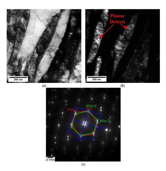
**Figure 14.** (a) Bright field (BF) TEM; (b) dark field (DF) TEM corresponding to  $\langle 110 \rangle \gamma$ ; (c) SAD patterns corresponding to  $[100]\alpha'1 \parallel [111]\alpha'2 \parallel [110]\gamma$  for M 675 °C + 120 s sample at  $\varepsilon$  = 0.10.
