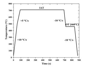
Figure 1. Schematic diagram of the heat treatment profile.
