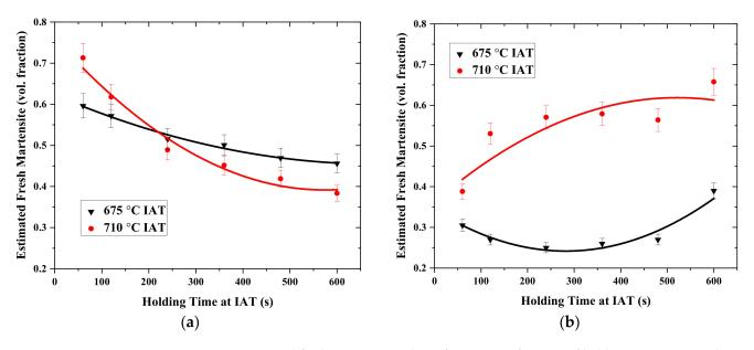
**Figure 6.** Estimated fresh martensite volume fraction as a function of holding time at 675 and 710 °C IATs for (**a**) CR and (**b**) M starting microstructures.
