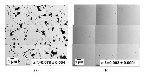
**Figure 4.** Montage of TEM micrographs showing carbide distribution in (**a**) CR and (**b**) M starting microstructures.
