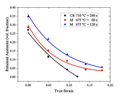
Figure 13. Retained austenite transformation kinetics for selected CR and M samples.
