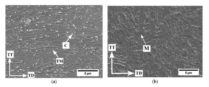
**Figure 3.** SEM micrographs of (**a**) as-received CR samples with tempered martensite and (**b**) heattreated M samples with martensite; C = carbides, TM = tempered martensite, M = martensite, TT = through thickness, TD = transverse direction.
