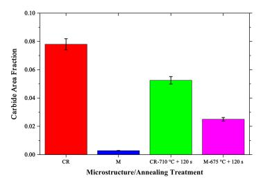
Figure 11. Carbide area fraction as a function of microstructure/heat treatment.
