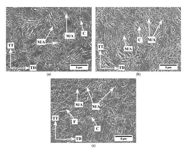
**Figure 8.** SEM micrographs of M samples annealed at 675 °C for (a) 120 s, (b) 360 s, (c) 600 s; C = carbide, F = ferrite, M = martensite, and A = retained austenite.
