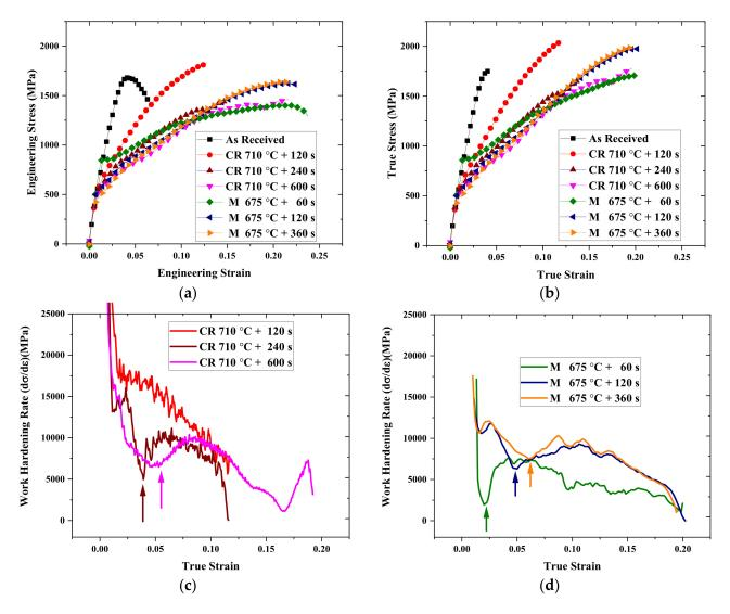
**Figure 12.** (**a**) Engineering stress vs. engineering strain; (**b**) true stress vs. true strain curves; work hardening rate vs. true strain curves for selected (**c**) CR and (**d**) M starting microstructures.
