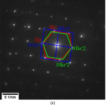
**Figure 9.** TEM results for the M 675 °C + 120 s sample: (a) Montage of bright field (BF) TEM micrographs; (b) dark field (DF) TEM corresponding to  $\langle 110 \rangle \gamma$ ; (c) SAD patterns corresponding to  $[100]\alpha'1 \parallel [111]\alpha'2 \parallel [110]\gamma$ .
