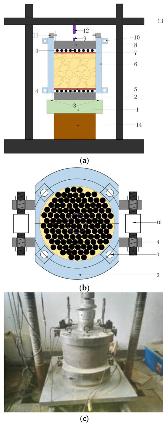
**Figure 1.** Test equipment (Note: 1—pedestal, 2—base, 3—load sensor, 4—steel ball, 5—the bottom force transmission plate, 6—semicircular rigid cylinders, 7—the top force transmission plate, 8—pressure plate, 10—tension sensors, 11—displacement sensor, 12—load sensor, 13—loading frame, and 14—loading device). (a) Sketch map of test equipment, (b) top view of the apparatus, and (c) physical view of the instrument.
