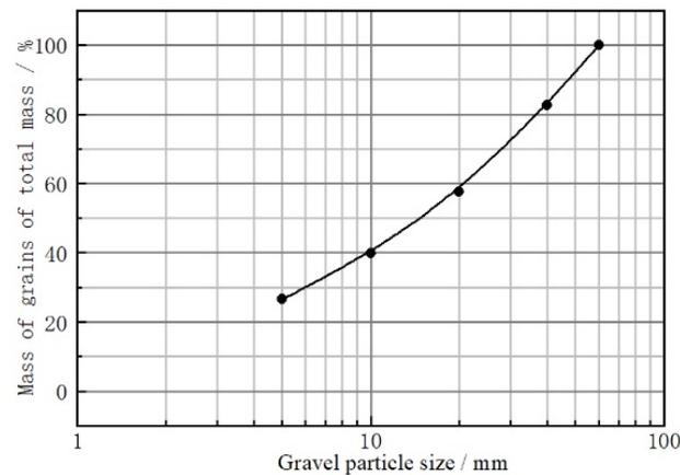
**Figure 2.** Particle Size Distribution (PSD) curves of test specimens.
