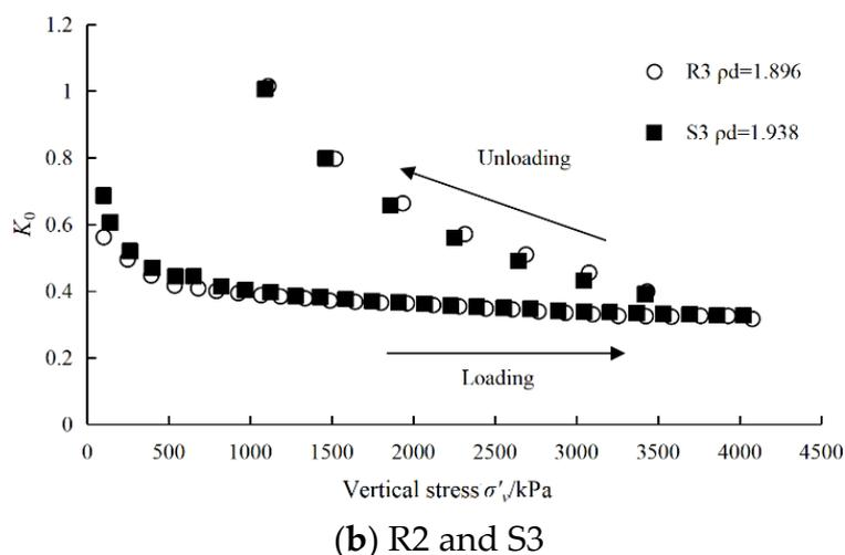
**Figure 8.**  $K_0$  behavior of sandy gravel and rockfill under loading and unloading conditions.
