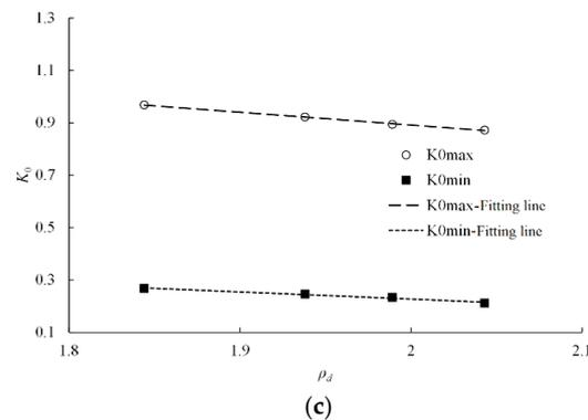
**Figure 4.**  $K_{0\max}/K_{0\min}-\rho_d$  fitting curves: (a) loading stage; (b) unloading stage. (c)  $K_{0\max}/K_{0\min}-D_{r0}$  fitting curves.
