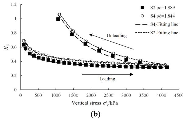
Figure 3.  $K_0$ - $\sigma_1$  curves with different  $p_d$ : (a) S1 and S3; (b) S2 and S4.
