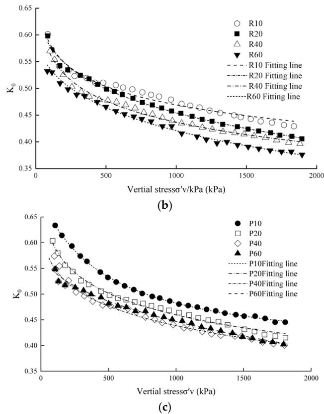
Figure 7.  $K_0$ – $\sigma'_v$  curves of the specimens for different techniques: (a) scalping technique, (b) replacement technique, and (c) parallel gradation technique.
