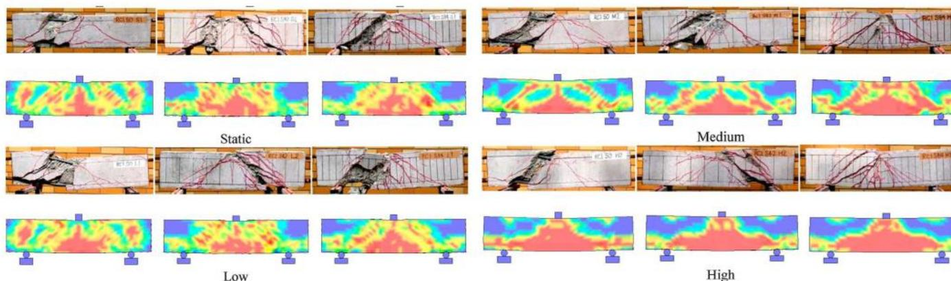
**Figure 10.** Comparisons between numerical and test results on cracking patterns for RC beam members under different loading rates [8].
