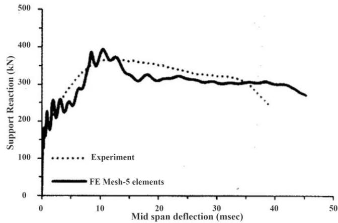
**Figure 13.** Comparison of experimental results and numerical simulations of mid-span deflection versus support reaction for RC beam [131].
