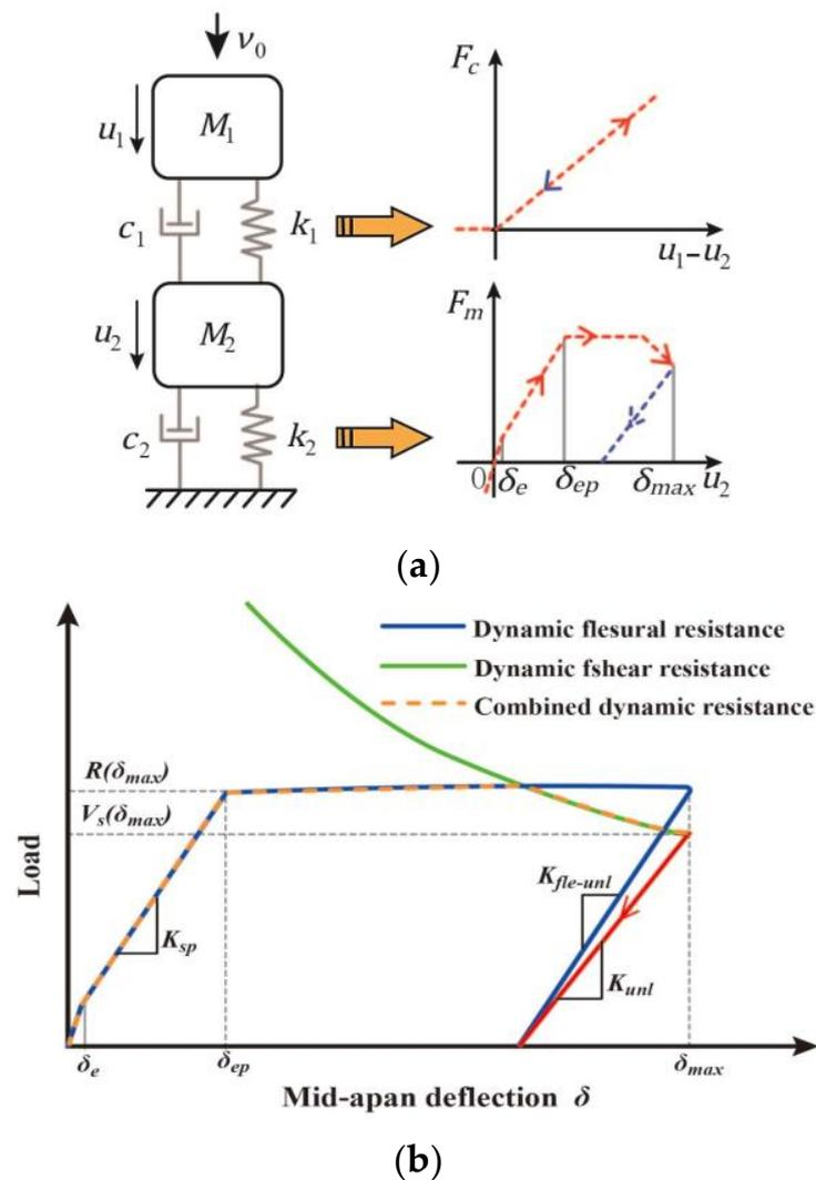
**Figure 14.** Schematic plot of 2DOF model for RC structural members considering the dynamic effect and different failure modes. (a) 2DOF numerical model; (b) Combined dynamic flexural and shear resistance function [137].
