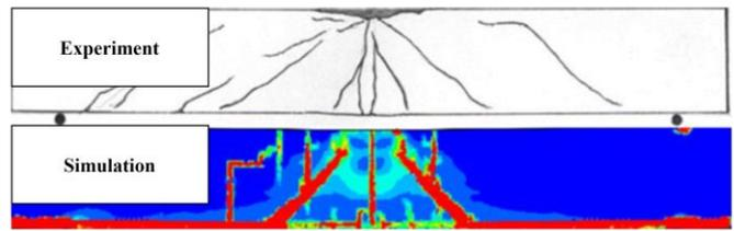
**Figure 12.** Failure patterns of RC beams obtained from tests and simulations [146].
