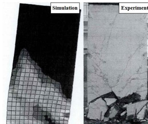
**Figure 9.** Damage to RC shear wall obtained from test and simulations [17].
