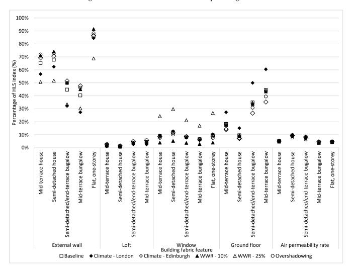
**Figure 11.** Significance of fabric sensitivity with varying climates, WWRs, and overshadowing compared to baseline.
