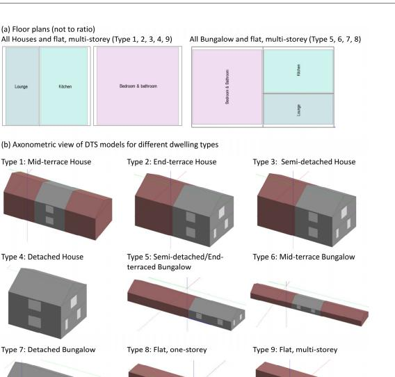
**Figure 2.** (a) Floor plan and (b) DTS models of three-bedroom building archetype for different dwelling types.
