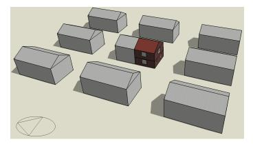
Figure 3. Model visualisations showing overshadowing from surrounding buildings.
