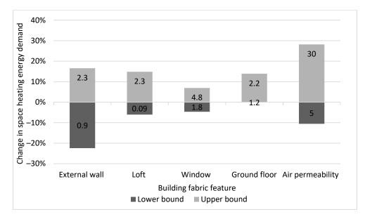
**Figure 6.** Percentage change relative to the base case for combined lower and upper bounds for five building fabric features, with the data labels showing the input parameters (U-values and air permeability) in Table 3.
