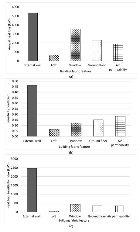
presented in Figure 5b indicates that the external wall rated most highly at 0.46, followed by the air permeability rate at 0.18, while the loft had the lowest coefficient at 0.065.
