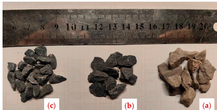
**Figure 1.** Aggregates: (a) black gravel with size of 5–10 mm; (b) black gravel with size of 10–15 mm; (c) Basalt stones with size of 10–20 mm.
