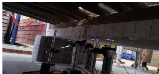
Figure 18. Positions of the displacement transducers.
