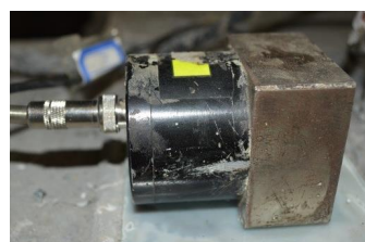
Figure 8. 891-II-type horizontal velocity sensors.
