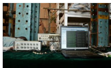
Figure 7. INV-306 intelligent signal acquisition processing analysis system.
