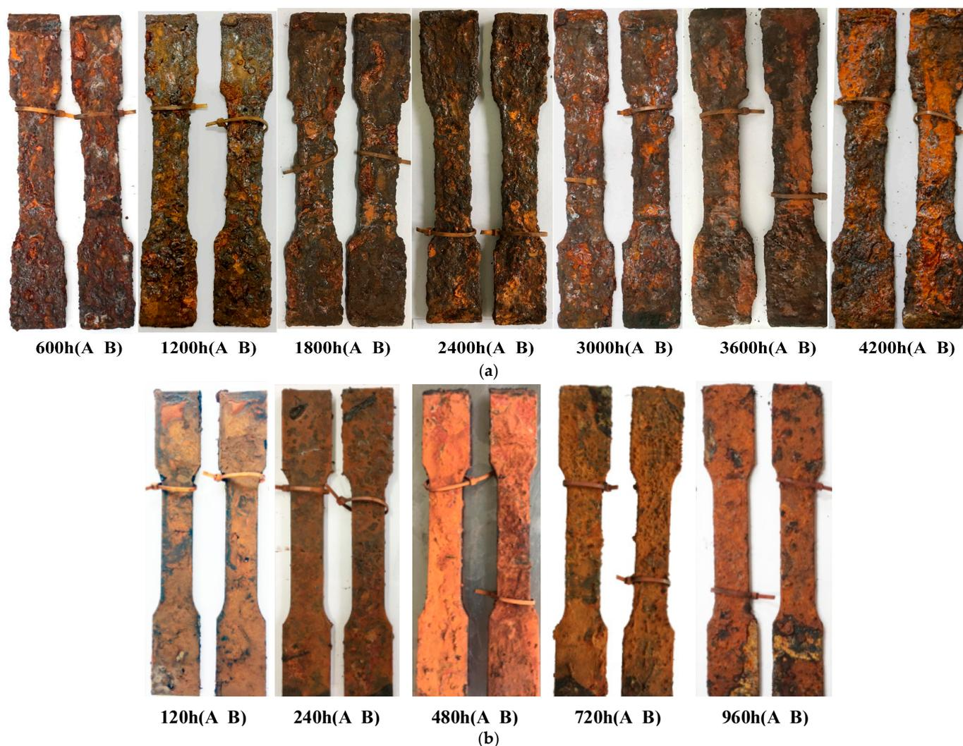
**Figure 2.** Morphologies of corroded specimens. (a) Specimens subjected to salt spray test; (b) specimens subjected to alternate immersion test.
