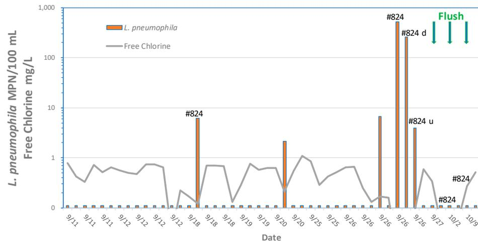
**Figure 13.** Impact of distribution system flushing at site 824 to control the occurrence of culturable *L. pneumophila*. Symbols: d, downstream of site 824; u, upstream of site 824. From LeChevallier [34].
