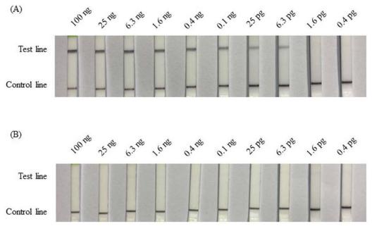
Figure 4. Molecular sensitivity test results for the RPA-LFD assay using 4-fold serially diluted total DNA extracted from pigeons as the template. (A) DNA template from a female pigeon. (B) DNA template from a male pigeon. In addition, a 100 ng, 25 ng, 6.3 ng, 1.6 ng, 0.4 ng, 0.1 ng, 25 pg, 6.3 pg, 1.6 pg, and 0.4 pg dilution series of total DNA was prepared from female and male pigeons.
