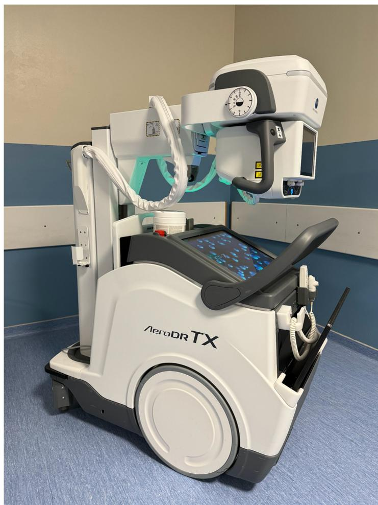
**Figure 1.** Mobile DDR equipment AeroDR TX m01 (manufactured by Sedecal, Madrid, Spain; distributed by Konica Minolta Business Solutions Europe GmbH, Hoofddorp, The Netherlands).
