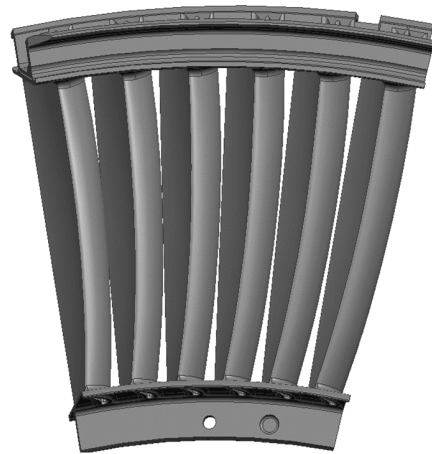
Figure 1. Nozzle guide vane of low-pressure turbine in aircraft engine.
