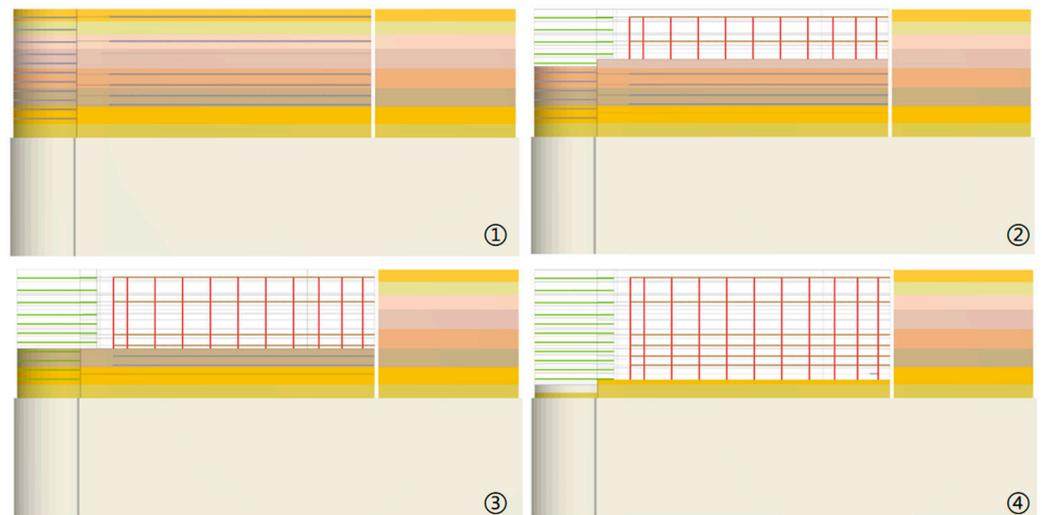
**Figure 8.** Schematic diagram of simultaneous excavation conditions.
