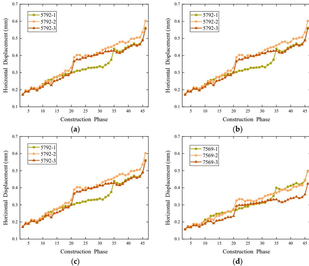
**Figure 12.** Comparison chart of horizontal displacement variation at various nodes for different excavation sequence scenarios. (a) Node: 61174, (b) Node: 5792, (c) Node: 59140, (d) Node: 7569.
