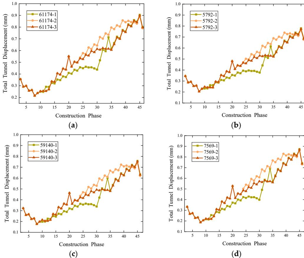
**Figure 13.** Comparison chart of total displacement variation at various nodes for different excavation sequence scenarios. (a) Node: 61174, (b) Node: 5792, (c) Node: 59140, (d) Node: 7569.
