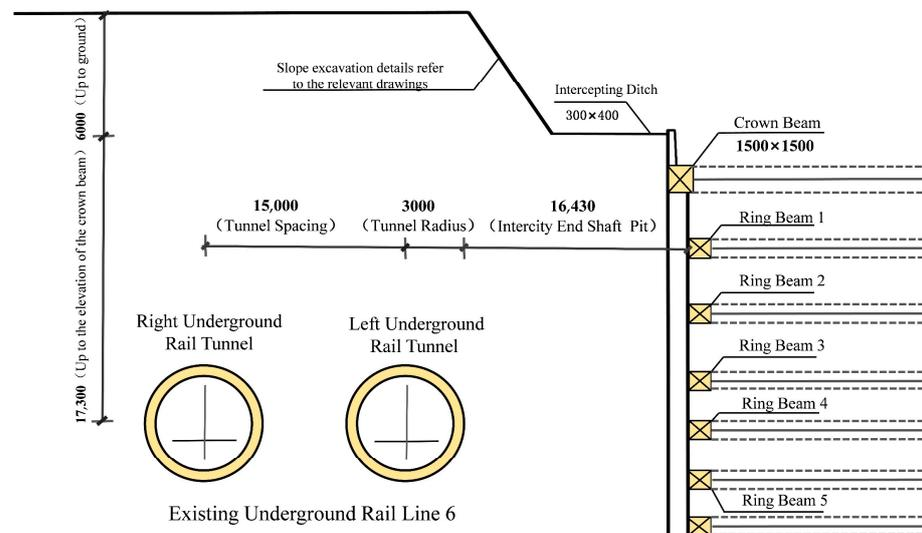
**Figure 3.** Relationship between the section position of the foundation pit and M6 line.
