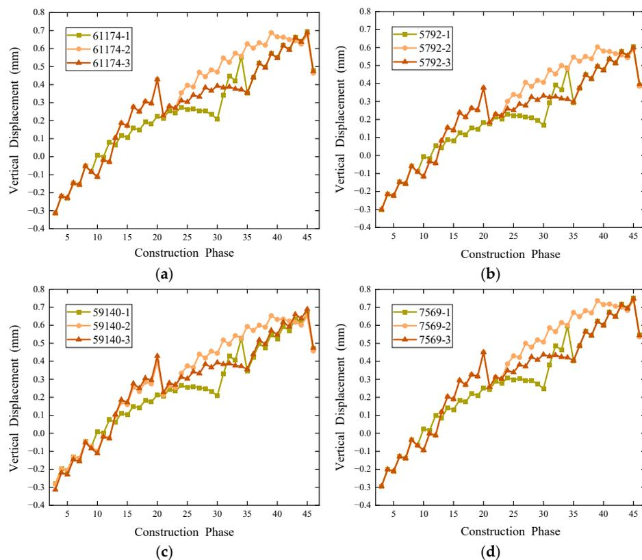
**Figure 11.** Comparison chart of vertical displacement variation at various nodes for different excavation sequence scenarios. (a) Node: 61174, (b) Node: 5792, (c) Node: 59140, (d) Node: 7569.
