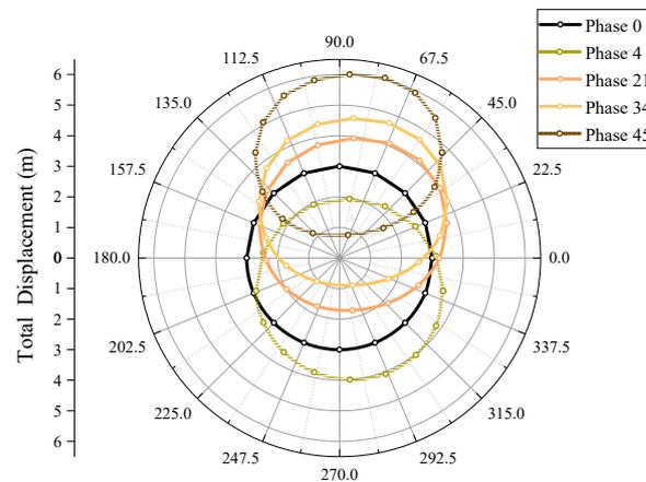
**Figure 14.** Under the comprehensive excavation plan the tunnel cross-section shifting trend.
