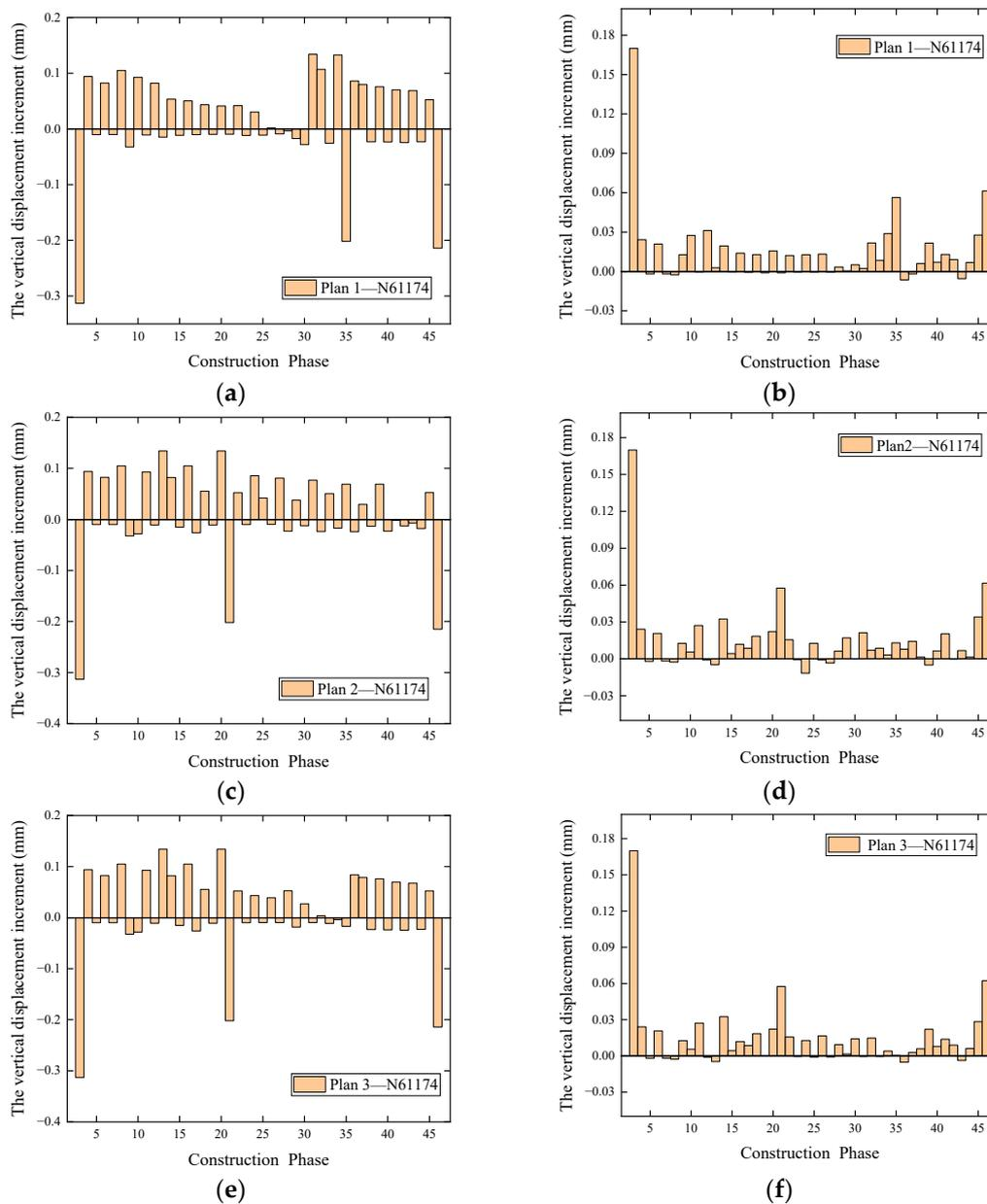
**Figure 15.** Vertical and horizontal displacement increment values for each scenario in each working condition. (a) P1: Incremental vertical displacement, (b) P1: incremental horizontal displacement, (c) P2: incremental vertical displacement, (d) P2: incremental horizontal displacement, (e) P3: incremental vertical displacement, (f) P3: incremental horizontal displacement.
