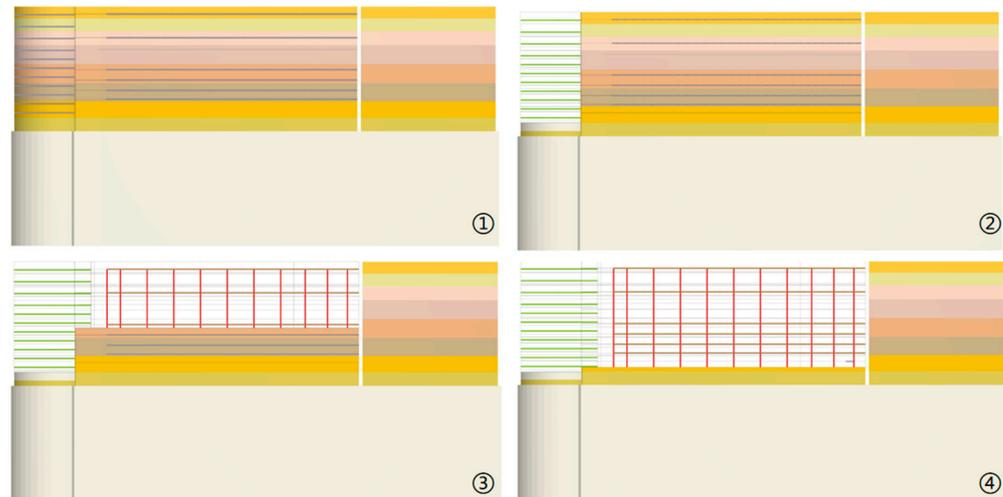
**Figure 7.** Schematic diagram of sequential excavation conditions.
