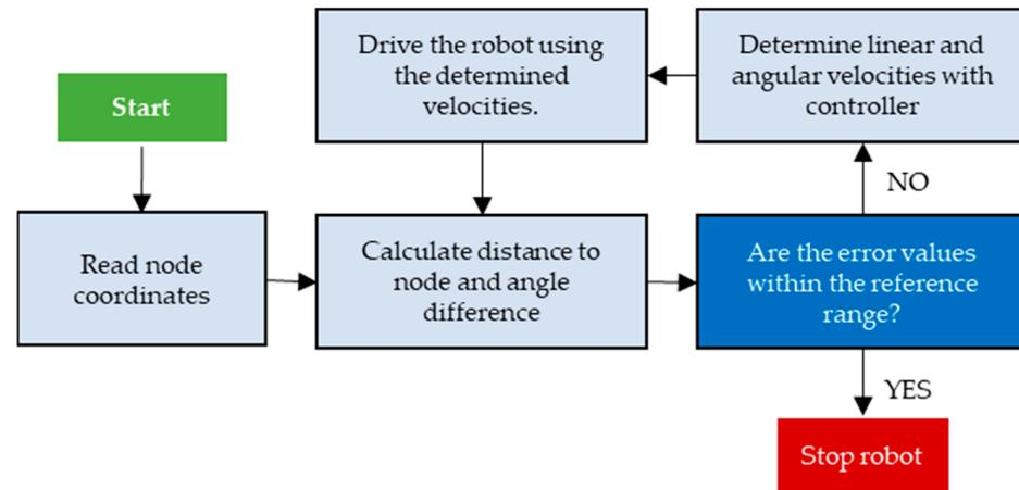
Figure 10. Block diagram of path tracking.
