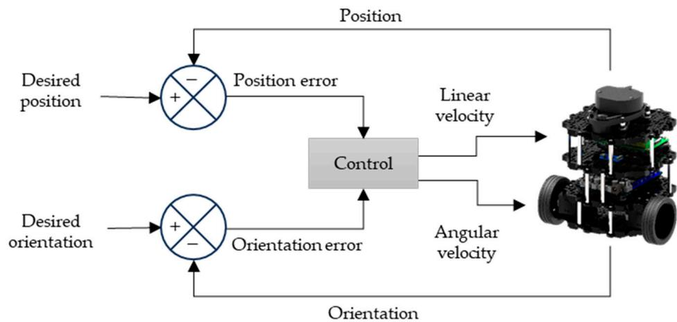
**Figure 8.** Block diagram of mobile robot control.
