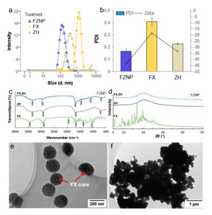
**Figure 1.** Characteristics of the fucoxanthin encapsulated with zein hydrolysate nanocomplex (FZNP). (a) The diameter, (b) zeta-potential and PDI, (c) Fourier transform infrared spectra and (d) X-ray diffraction of FZNP, the wall material zein hydrolysate (ZH) and free fucoxanthin (FX). (e) The TEM image of FZNP and (f) free FX solution. (c–f) were cited from the results of Zhang et al. (2022) (Reprinted with permission from Ref. [24]. 2022, Elsevier).
