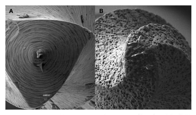
**Figure 8.** (**A**) Scanning Environmental Microscope image of the tip of a Grinded Niti file. (**B**) Scanning Environmental Microscope image of the tip of an Electrical Discharge Machined Niti file. The EDM procedure creates a rough surface in the tip of the instrument, making the tip active when activated and increasing the cutting efficiency of the file (images courtesy of Dr. Alexey Volokitin, city of Dnepr, Ukraine).
