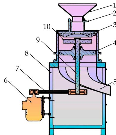
**Figure 15.** The structure of flaxseed dehulling equipment: (1) hopper; (2) feeding control board; (3) fixed table; (4) fixed device of transmission shaft; (5) outlet port; (6) motor; (7) belt; (8) stand; (9) transmission shaft; (10) dynamic table.
