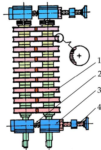
**Figure 7.** Roller structure: (1) extrusion rollers; (2) compression spring; (3) bearing seat; (4) adjusting screws.
