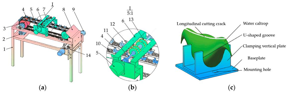
**Figure 5.** Clamping-type fresh water chestnut dehulling machine: (a) horizontal cutting and dehulling device; (b) local enlargement; (c) clamping-type device; (1) frame; (2) pulley I; (3) chain wheel; (4) baseplate; (5) transversal cutting motor; (6) beam; (7) transversal cutting blade; (8) retaining plate; (9) rubber roller motor; (10) chain; (11) blade shaft; (12) elastic strip; (13) transversal cutting blade; (14) rubber roller.
