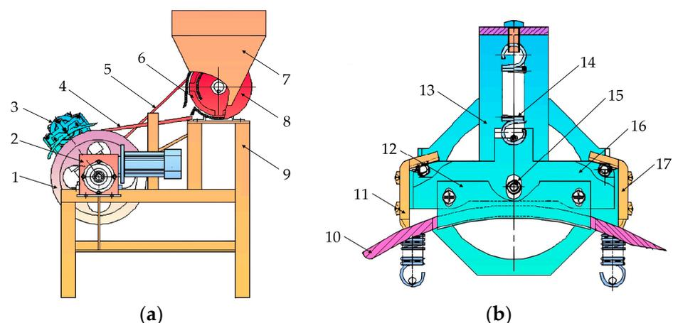
**Figure 8.** Schematic of lotus seed sheller: (a) overall structure diagram; (b) suspended vibratory dehulling mechanism; (1) driving wheel; (2) speed regulating motor; (3) suspended vibratory dehulling device; (4) chute; (5) V-belt; (6) hopper; (7) discharge wheel; (8) discharge wheel cover; (9) frame; (10) pressing plate; (11) left guide rail; (12) blade; (13) spring fixing plate; (14) spring; (15) eccentric pin; (16) blade holder; (17) right guide rail.
