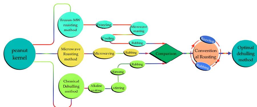
**Figure 9.** Process flow of removing seed coat from peanut kernels.
