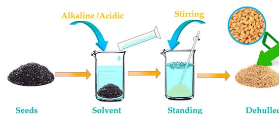
**Figure 1.** Chemical dehulling principle.
