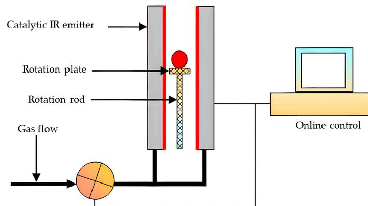
**Figure 14.** Principle of infrared tomato peeling.
