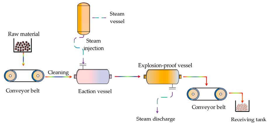
**Figure 10.** Steam explosion dehulling principle.
