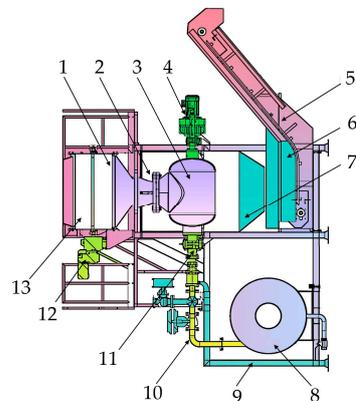
**Figure 11.** Structure diagram of steam sheller: (1) separator; (2) discharge port; (3) steam reaction tank; (4) motor; (5) mesh belt conveyor; (6) collection pond; (7) discharge port; (8) steam tank; (9) rack; (10) pipeline; (11) rotary joint; (12) gear motor; (13) driveshaft.
