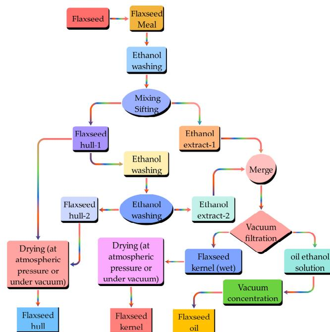
**Figure 2.** Ethanol dehulling process of flaxseed.
