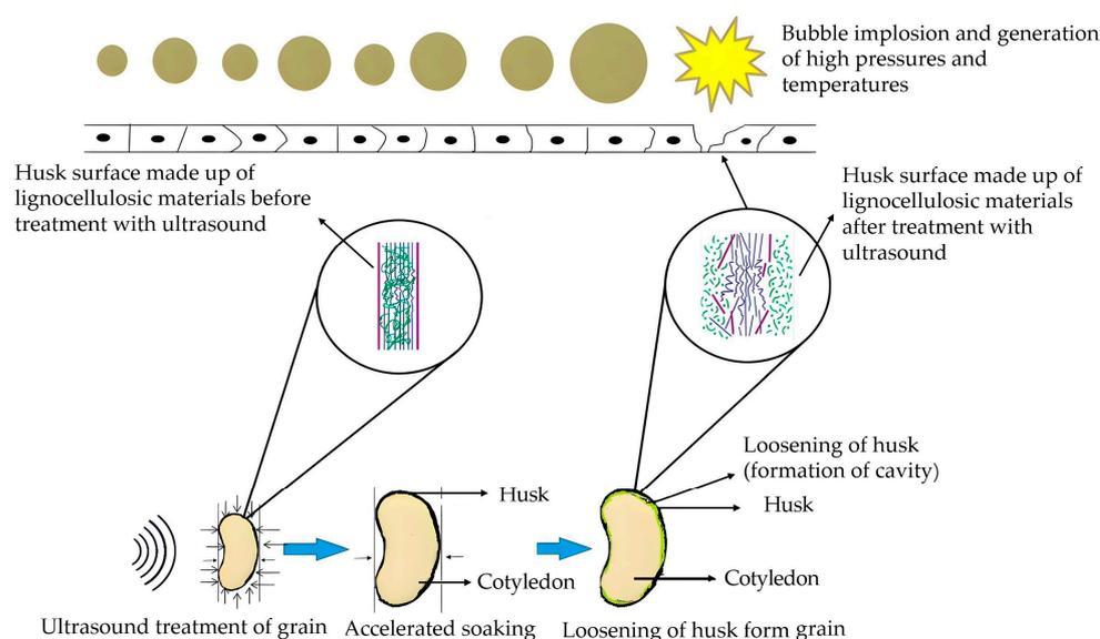
**Figure 12.** Ultrasonic dehulling principle.
