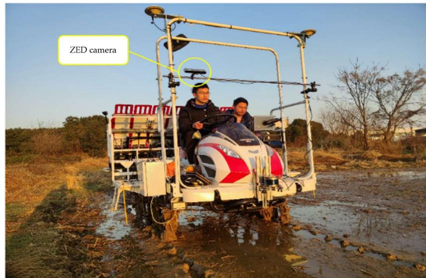
**Figure 1.** Data acquisition platform.
