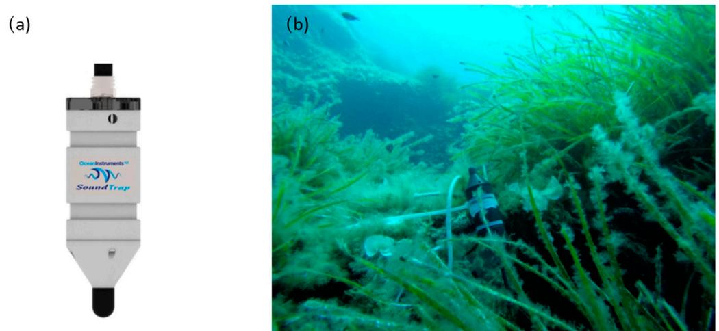
**Figure 5.** (a) Image of SoundTrap ST300 hydrophone used; (b) Image of the hydrophone deployed on seafloor in Ċirkewwa, amidst the *Posidonia* meadows.
