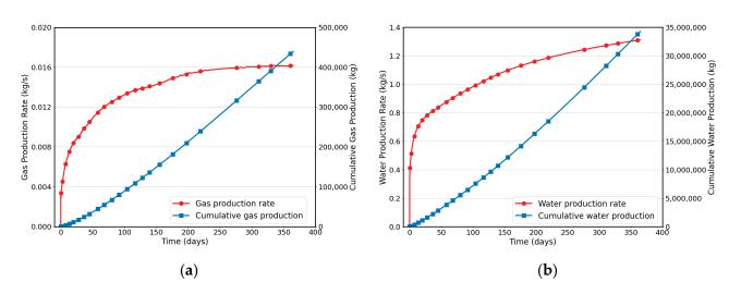
Figure 5. Gas (a) and water (b) production over time during the 365-day production test.
