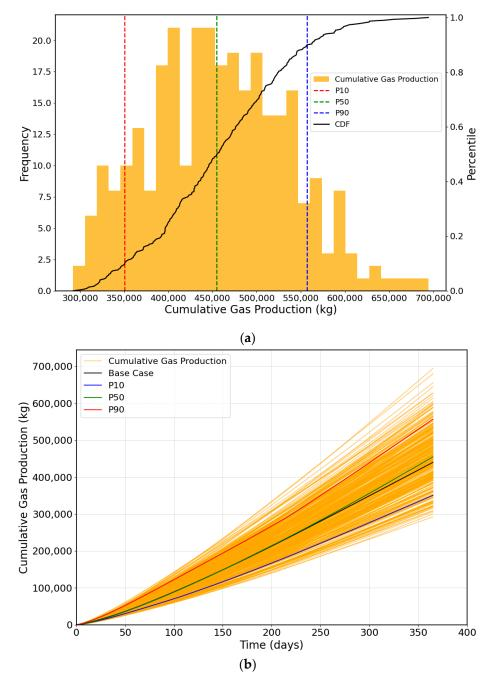
**Figure 8.** Results of uncertainty analysis conducted on 300 cases of cumulative gas production. (a) Histogram, alongside the percentiles for cumulative gas production after 1 year and (b) cumulative gas production.
