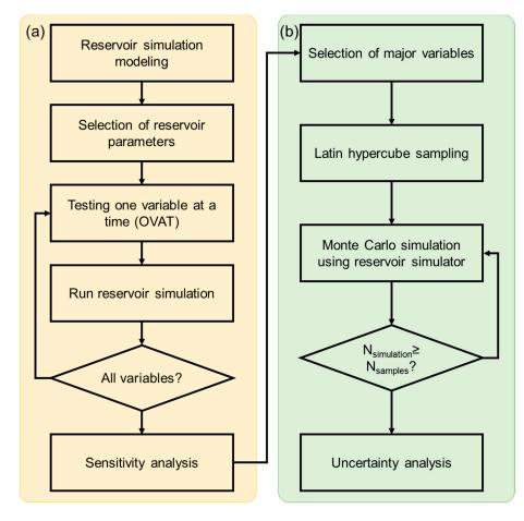
**Figure 1.** Methodology for sensitivity and uncertainty analysis in gas hydrate reservoirs. (**a**) Performing sensitivity analysis on all selected reservoir parameters using the one-variable-at-a-time (OVAT) approach; (**b**) selecting major variables with high sensitivity and analyzing reservoir property uncertainty through Latin hypercube sampling-based Monte Carlo simulation.
