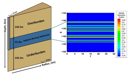
**Figure 2.** Schematic diagram of the cylindrical system(**left**) and initial gas hydrate saturation distribution (**right**) in the UBGH2-6 reservoir.
