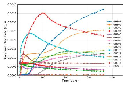
Figure 6. Gas production rate of each layer during the 365-day production test.
