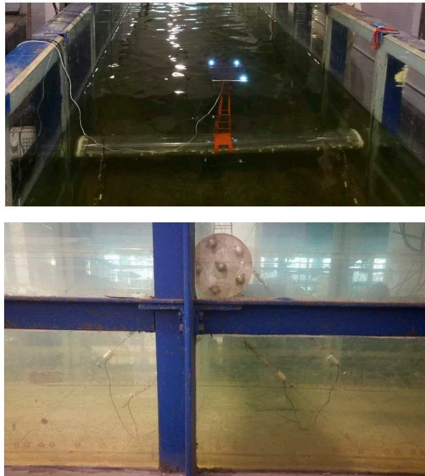
Figure 3. The model SFT moored in test tank.
