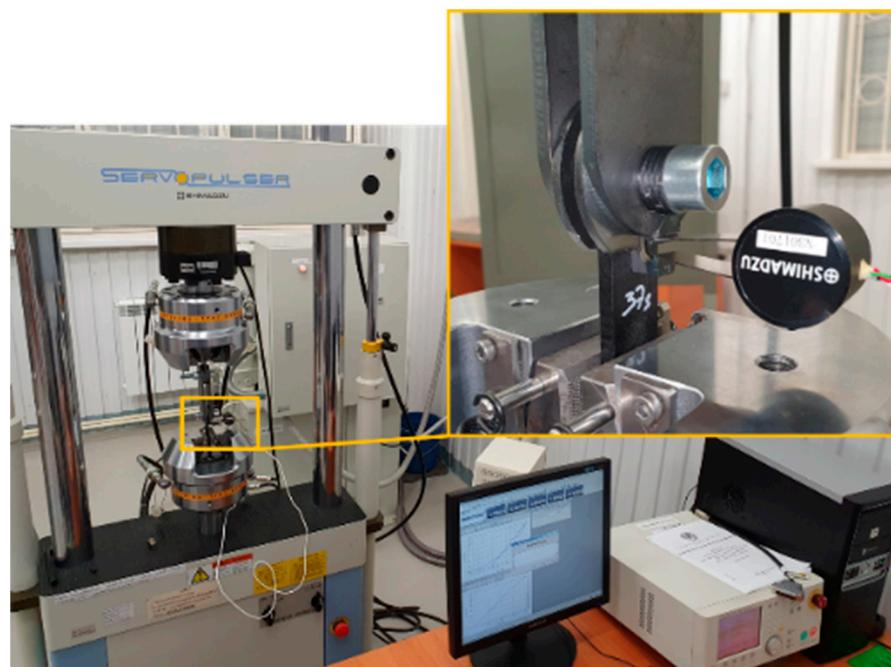
**Figure 21.** Test to determine the load-bearing capacity of lugs.
