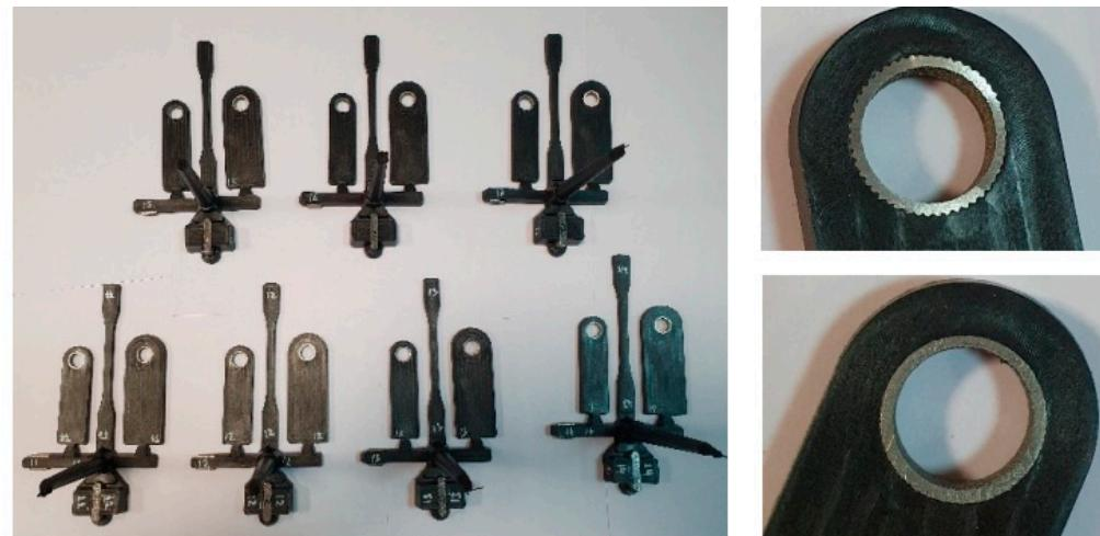
**Figure 12.** Manufactured lugs.
