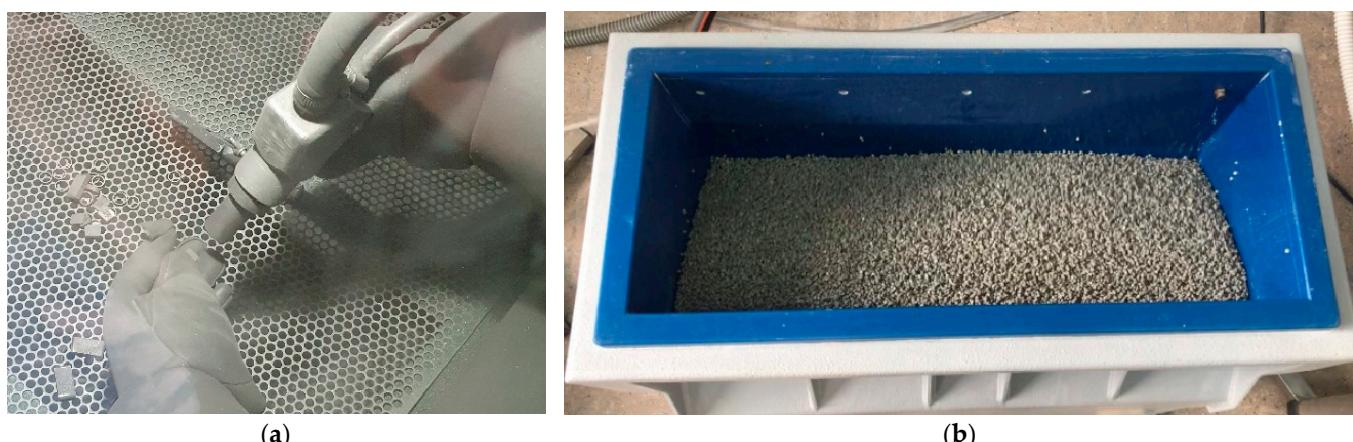
**Figure 6.** The roughness: (a) sandblasting, (b) vibratory finishing.
