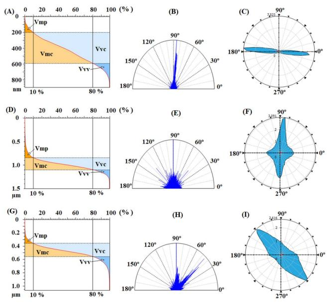
**Figure 7.** Abbott–Firestone curves with functional volume parameters, texture direction representations and graphs with polar coordinates to analyze orientation with azimuth angle obtained for rubbed EPI-pBAPS (1R) (A–C), EPI-pBAPS (2R) (D–F) and EPI-pBAPS (3R) (G–I) samples.
