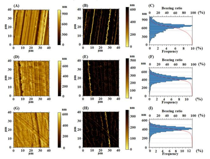
**Figure 8.** 2D topographical images, furrow maps and histograms/Abbott curves obtained for rubbed CBDA-pBAPS (1R) (**A–C**), CBDA-pBAPS (2R) (**D–F**) and CBDA-pBAPS (3R) (**G–I**) samples.
