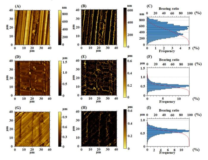
**Figure 6.** 2D topographical images, furrow maps and histograms/Abbott curves obtained for rubbed EPI-pBAPS (1R) (**A–C**), EPI-pBAPS (2R) (**D–F**) and EPI-pBAPS (3R) (**G–I**) samples.
