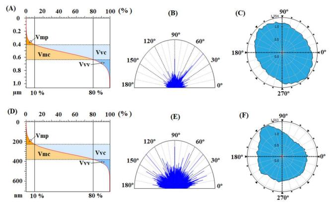
**Figure 11.** Abbott–Firestone curves with functional volume parameters, texture direction representations and graphs with polar coordinates to analyze orientation with azimuth angle obtained for DBD plasma-treated rubbed EPI-pBAPS (3R) (**A**–**C**) and CBDA-pBAPS (3R) (**D**–**F**) samples.
