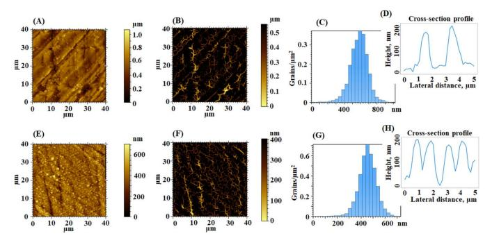
**Figure 10.** 2D topographical images, furrow maps, grains distribution and grains cross-section profiles obtained for plasma-treated rubbed EPI-pBAPS (3R) (**A**–**D**) and CBDA-pBAPS (3R) (**E**–**H**) samples.
