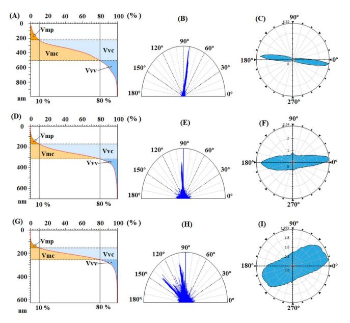
**Figure 9.** Abbott–Firestone curves with functional volume parameters, texture direction representations and graphs with polar coordinates to analyze orientation with azimuth angle obtained for rubbed CBDA-pBAPS (1R) (**A**–**C**), CBDA-pBAPS (2R) (**D**–**F**) and CBDA-pBAPS (3R) (**G**–**I**) samples.
