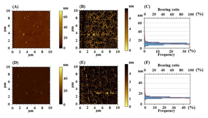
**Figure 4.** 2D topographical images, furrow maps and histograms/Abbott curves obtained for pristine EPI-pBAPS (**A**–**C**) and pristine CBDA-pBAPS (**D**–**F**) samples.
