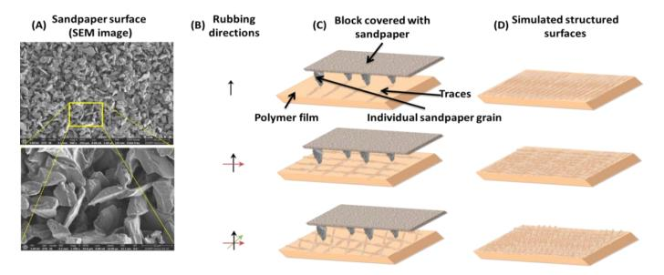
**Figure 1.** Illustration of the rubbing process: **(A)** SEM images of the sandpaper evidencing the individual grains layout and appearance. The yellow box represents the zone where the sandpaper was scanned at higher magnitude; **(B)** rubbing directions; **(C)** schematic representation of the rubbing device; **(D)** simulated structured polymer surfaces.
