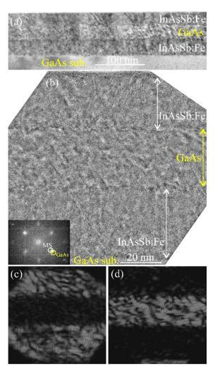
InAsSb:Fe layer. Note that the lattice mismatch between the GaAs and InSb amounts to 14.6 % and between the GaAs and InAs to 7.2 %.
