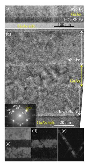
Figure 7. Cross-section TEM images of the InSb:Fe/GaAs/InGaSb:Fe/GaAs (sub.) structure of M3.
