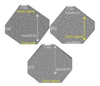
**Figure 5.** Cross-section HRTEM images of each layer of sample M2. (**a**) HRTEM image of the lower InAsSb:Fe layer. (**b**) HRTEM image of the GaAs spacer. (**c**) HRTEM image of the upper InGaSb:Fe layer.
