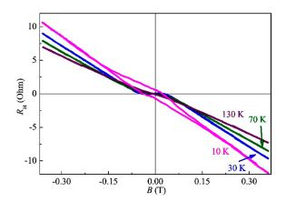
**Figure 11.**  $R_{\rm H}(B)$  dependences at various temperatures for sample S1.
