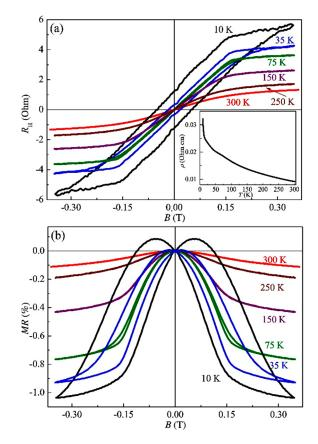
**Figure 13.**  $R_{\rm H}(B)$  dependences (**a**) and magnetoresistance (**b**) at various temperatures for sample S3.
