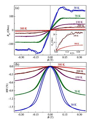
Figure 12.  $R_{\rm H}(B)$  dependences (a) and magnetoresistance (b) at various temperatures for sample S2.
