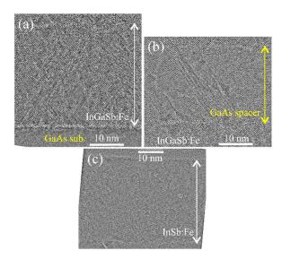
**Figure 8.** Cross-section HRTEM images of each layer of sample M3. (**a**) HRTEM image of the lower InGaSb:Fe layer. (**b**) HRTEM image of the GaAs spacer. (**c**) HRTEM image of the upper InSb:Fe layer.
