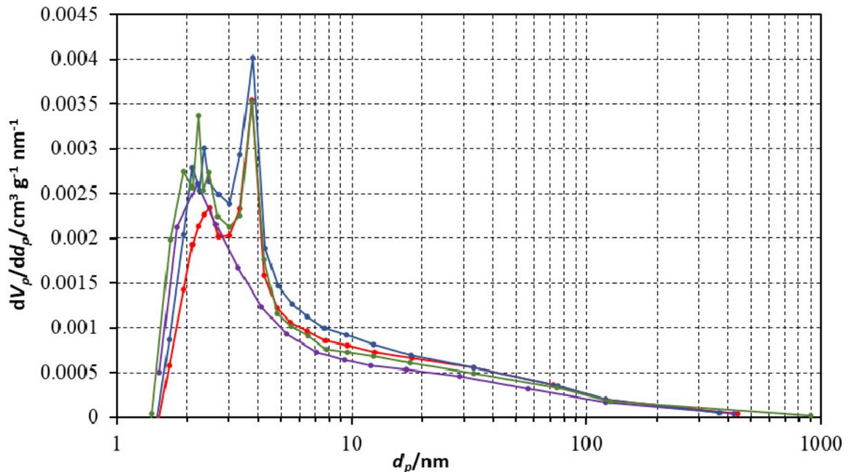
**Figure 7.** Pore size distribution of PGs and NG. — NaG; — PG<sub>Bel</sub>; — PG<sub>Bal</sub>; — PG<sub>Kin</sub>.
