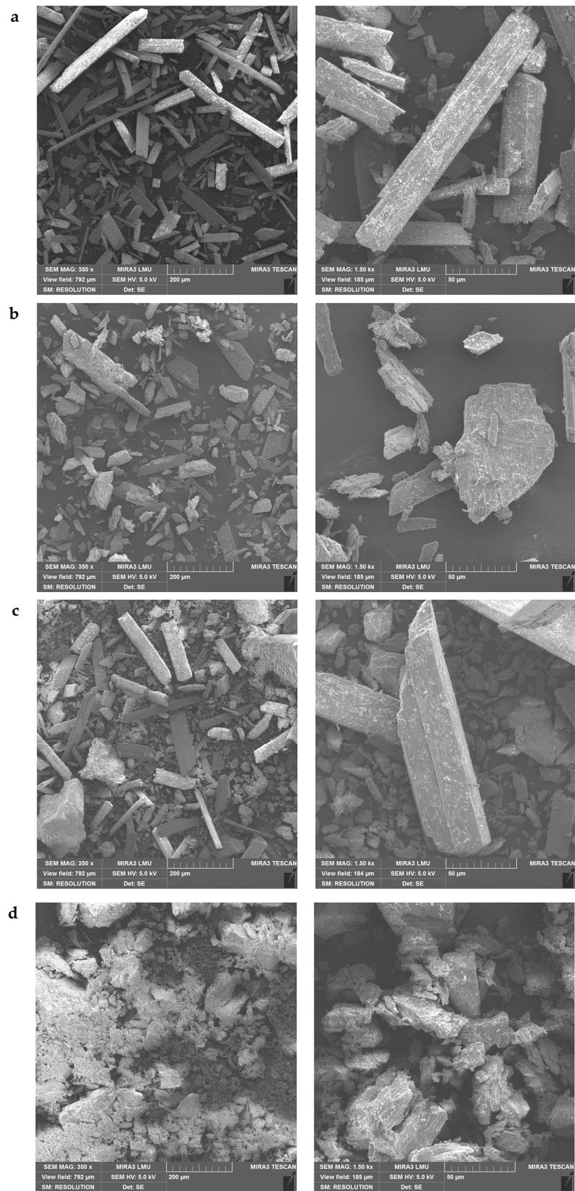
Figure 8. Morphology of the binder based on: (a)—PG<sub>Bel</sub>; (b)—PG<sub>Bal</sub>; (c)—PG<sub>Kin</sub>; (d)—NG.
