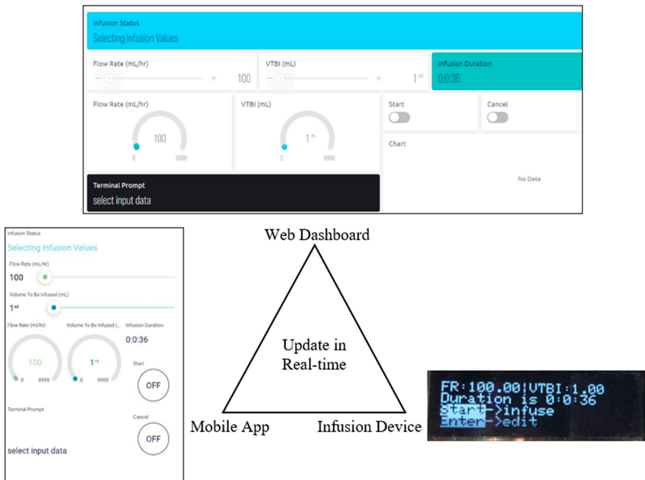
Figure 22. IoT real-time performance test.
