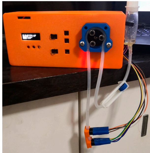
Figure 20. Physical design of the IoT-based automated drug infusion device.
