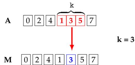
**Figure 5.** Movmean function in Matlab package. A window ( $k$ ) reveals the number of arrays that were taken to calculate the average neighboring elements.
