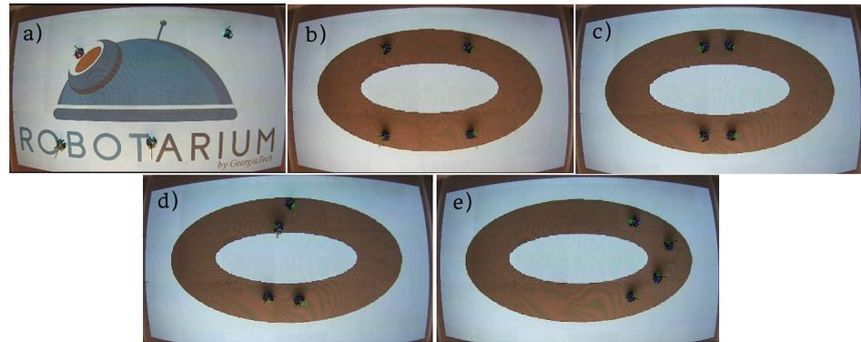
**Figure 11.** Robotarium experimental simulation, implemented into GRITSBot-X: (a) start of the experiment, (b) positioning of robots, (c) start of collision avoidance algorithm, (d) collision avoidance procedure, and (e) robots are in the middle of the track and follow each other.
