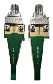
Figure 5. Near-field electric- and magnetic-field probes.
