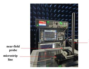
Figure 10. Near-field scanning diagram.
