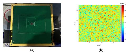
Figure 13. Near-field acquisition: (a) HKA32133 test board; (b) field strength distribution.
