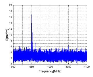
Figure 12. Electric field strength diagram of high-voltage charging pile.
