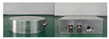
Figure 4. Pulsed electric-field probe and photoelectric converter.
