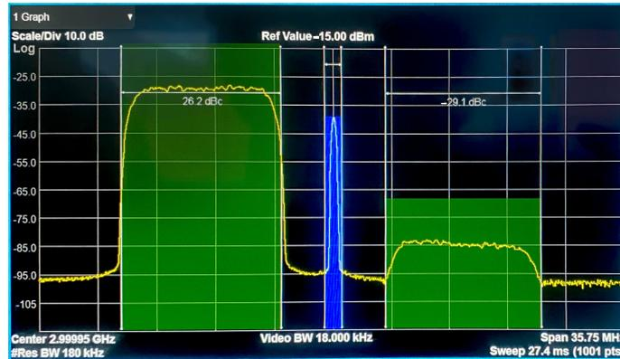
**Figure 12.** The digital calibration results with a symbol transmission rate of 8 Msps quadrature phase shift keying (QPSK) signal and a 3.0 GHz center frequency. The IRR was 55.3 dBc.
