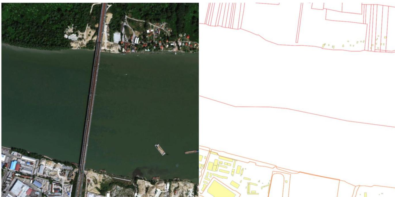
**Figure 8.** An example of weak data completeness quality (no geometric data about the bridge) [39].
