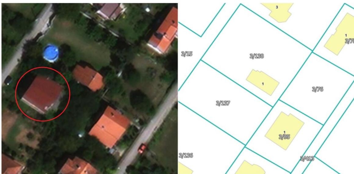
**Figure 10.** An example of weak data timeliness quality—no data on a building (red circle) constructed several years ago [39].
