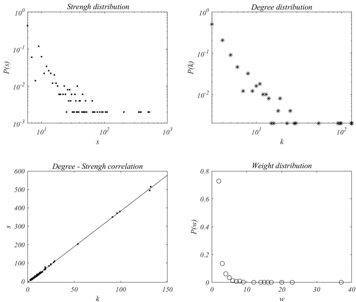
**Figure 4.** The distribution characteristics of the BBV network. The degree distribution, node strength distribution, and weight distribution of the BBV network all conform to the power-law distribution, and the degree and strength of the nodes have a positive correlation.
