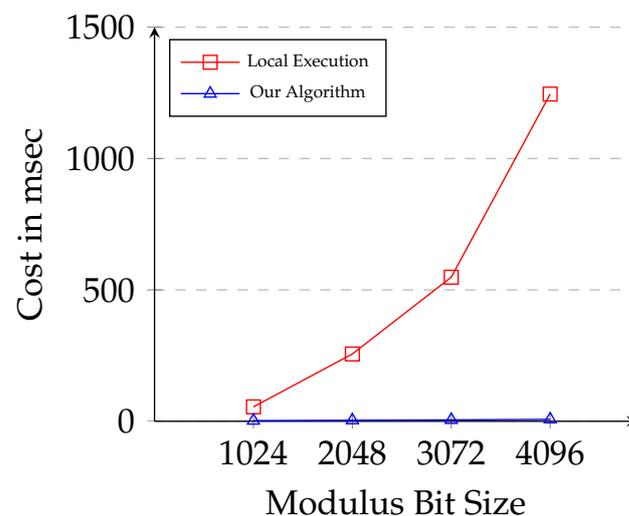
**Figure 1.** Local execution (without outsourcing) vs. using our algorithm (with outsourcing).
