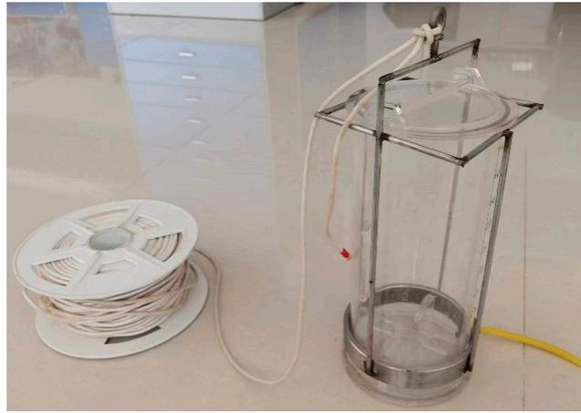
Figure 5. Hand-thrown sampler.
