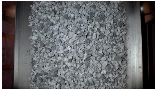
**Figure 5.** Example of an acquired image of coke on the conveyor belt.
