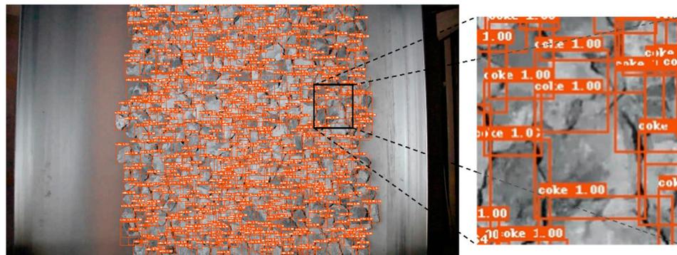
Figure 8. Image of the results of the coke particle detection model, with coke particles marked by orange bounding boxes.
