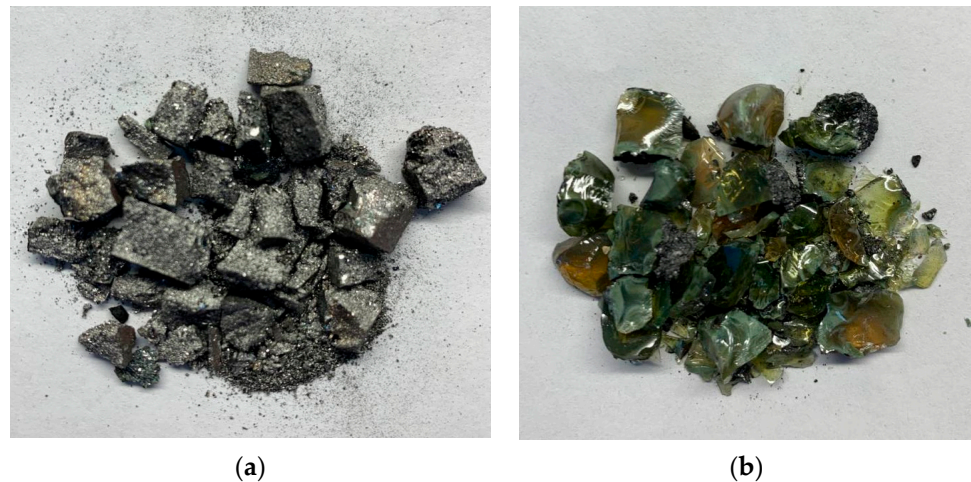
Figure 2. Ferrosilicomanganese melting products: (a) alloy; (b) slag.
