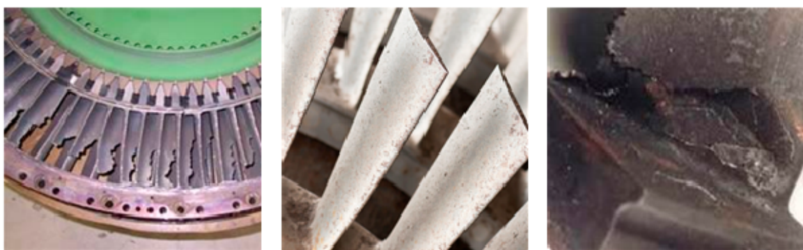
Figure 5. Physical diagram of turbine blade failure.
