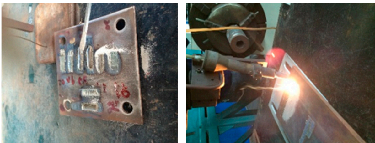
Figure 12. Laser cladding remanufacturing of turbine blade.
