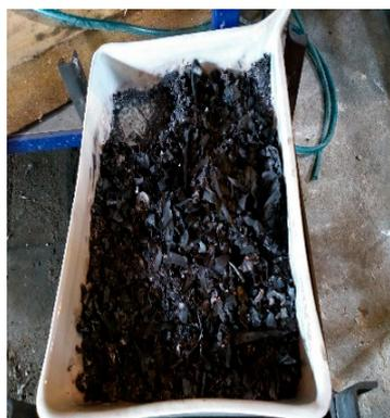
Figure 1. Solid WPCB material after thermal pre-treatment.
