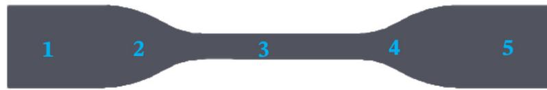
**Figure 7.** Surface roughness measurement on the selected five points of the top surface of tensile specimens [48].
