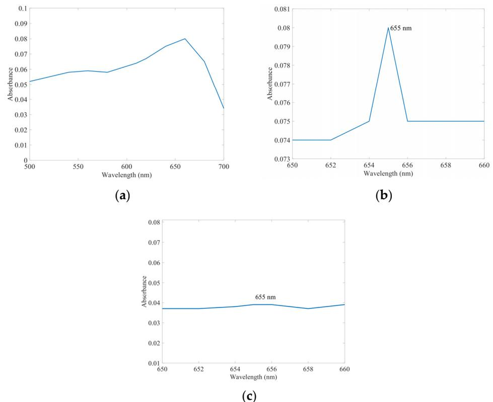
**Figure 2.** The real textile wastewater's (WW's) absorbance spectra. (a) The absorbance spectrum in a wide range of wavelengths, (b) the absorbance spectrum in a smaller wavelength range, and (c) the absorbance spectrum after adsorption with *Pinus patula* BC.
