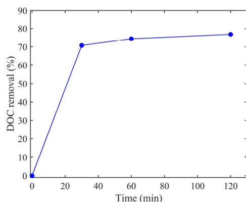
**Figure 4.** Dissolved organic carbon (DOC) removal vs. time. Operational conditions: BC dose = 13.5 g/L, pH = 3, BC particle size = 300–450  $\mu\text{m}$ .
