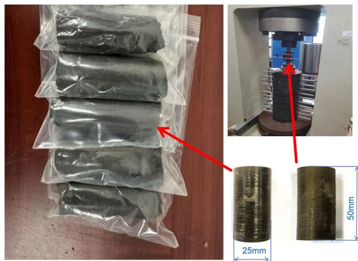
**Figure 1.** Uniaxial compressive strength test.
