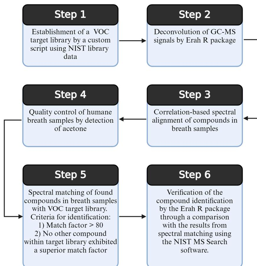
**Figure 3.** A flowchart of the custom GC-MS analysis R script, which utilizes the ERAH package. Figure created with [BioRender.com](https://www.biorender.com).
