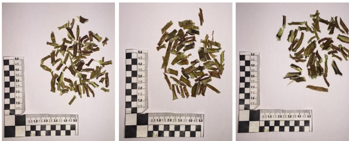
Figure 10. Purslane twigs after drying. From the left: at 2.3 kW—20 min; at 1.15 kW—30 min; at 0.46 kW—50 min.
