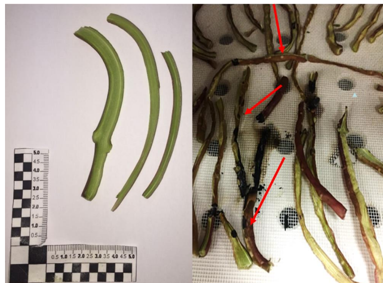
Figure 8. Purslane fresh-cut twigs (on the left); burned purslane twigs after preliminary drying test at 2.3 kW (on the right). The red arrows indicate the burn effects due to dissipation mechanisms.
