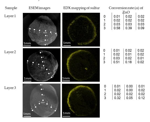
**Figure 6.** ESEM pictures and elemental mapping obtained for yellow particles of transformed sorbent from packed bed scale process at 300  $^{\circ}$ C.
