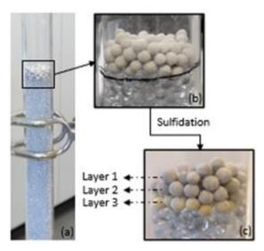
**Figure 3.** Photographs of the sorbent; (a) in the reactor supported by glass beads before sulfidation; (b) close-up view of the sorbent; (c) after sulfidation with the three layers selected along the packed bed height.
