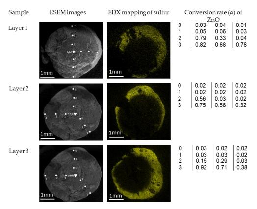
**Figure 5.** ESEM pictures and elemental mapping obtained for dark grey particles of transformed sorbent from packed bed scale process at 300  $^{\circ}$ C.
