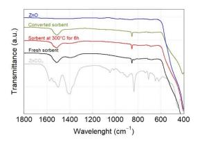
**Figure 7.** Fourier Transform Infrared—Attenuated Total Reflectance (FTIR-ATR) spectra of the fresh, thermally treated at 300 °C for 6 h and converted Hi-Fuel A310 sorbents from packed bed scale process compared with pure compounds: ZnO and ZnCO<sub>3</sub>.
