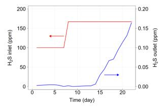
**Figure 2.** Breakthrough curve for 0.8 cm height Hi-Fuel sorbent at 300 °C with the injection of 100 ppm  $H_2S$  for 7 days followed by 167 ppm  $H_2S$  for 15 days. Gas flow of mixture  $H_2S/N_2$ —60 NmL/min (GHSV = 637 h<sup>-1</sup>).
