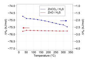
Figure 10. Enthalpy difference calculated for sulfidation reactions of ZnO and ZnCO<sub>3</sub>.
