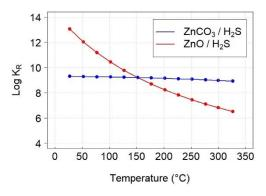
Figure 12. Equilibrium constant (K<sub>R</sub>) calculated for sulfidation reactions of ZnO and ZnCO<sub>3</sub>.
