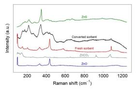
**Figure 9.** Raman spectra of the fresh and converted sorbents Hi-Fuel compared with pure compounds:  $ZnO_3$  and ZnS.
