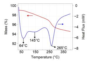
**Figure 8.** Thermogravimetric Analysis/Differential Scanning Calorimetry (TGA/DSC) of the fresh sorbent Hi-Fuel. ( $m_0 = 36.62 \text{ mg}$ ).
