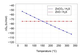
**Figure 11.** Gibbs energy ( $\Delta G_R$ ) calculated for sulfidation reactions of ZnO and ZnCO<sub>3</sub>.
