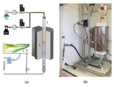
**Figure 1.** (a) Schematic view; (b) and picture of the experimental setup used for the sulfidation tests. 1—mass flow meter, Brooks Instrument; 2—glass reactor with an internal diameter of 3 cm; 3—tube furnace; 4—sampling nozzle providing a flow rate of about 3 L/h through the AP2E analyzer; 5—AP2E analyzer; 6—AP2E analyzer pump.
