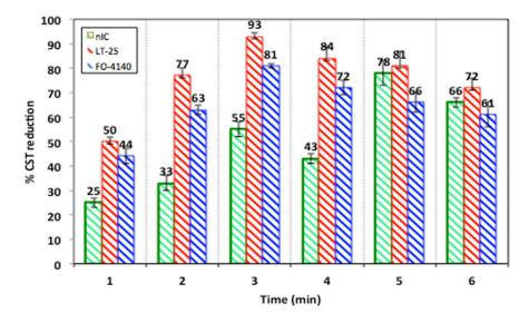
Figure 4. CST reduction efficiency of various conditioners at various conditioning times.
