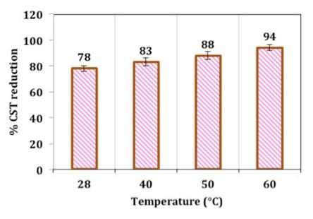
Figure 9. CST reduction efficiency linked to temperature effect using nIC-Conditioner/H<sub>2</sub>O<sub>2</sub>.
