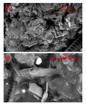
**Figure 5.** SEM images of "(**A**)" raw sludge and "(**B**)" sludge conditioned using the nIC-Conditioner catalyst composite.
