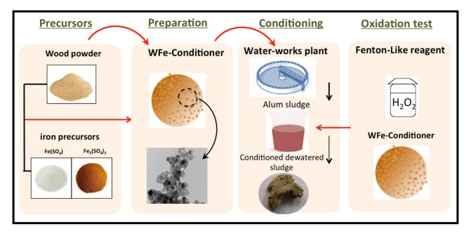
was analyzed using a capillary suction time (CST) test. Figure 1 demonstrates a schematic graphical illustration of the experimental steps.
