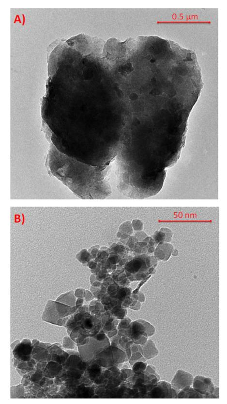
Figure 3. TEM images of "(A)" pristine cellulose and "(B)" nIC-Conditioner catalyst composite.
