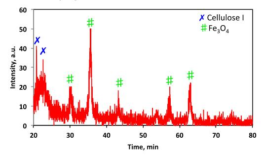
Figure 2. X-ray diffraction patterns of the nIC-Conditioner catalyst composite.
