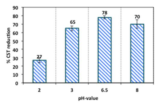
Figure 8. CST reduction efficiency linked to sludge pH using nIC-Conditioner/H<sub>2</sub>O<sub>2</sub>.
