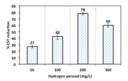
Figure 7. CST reduction efficiency at various hydrogen peroxide doses.
