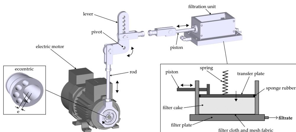
**Figure 2.** Apparatus developed by Illies et al. [30] for filter cake compaction by oscillatory shear at a low compressive pressure at a laboratory scale. The figure is from Yildiz et al. [33], reprinted with the permission of the publisher (Taylor & Francis Ltd., <http://www.tandfonline.com>, accessed on 23 Januar 2024).
