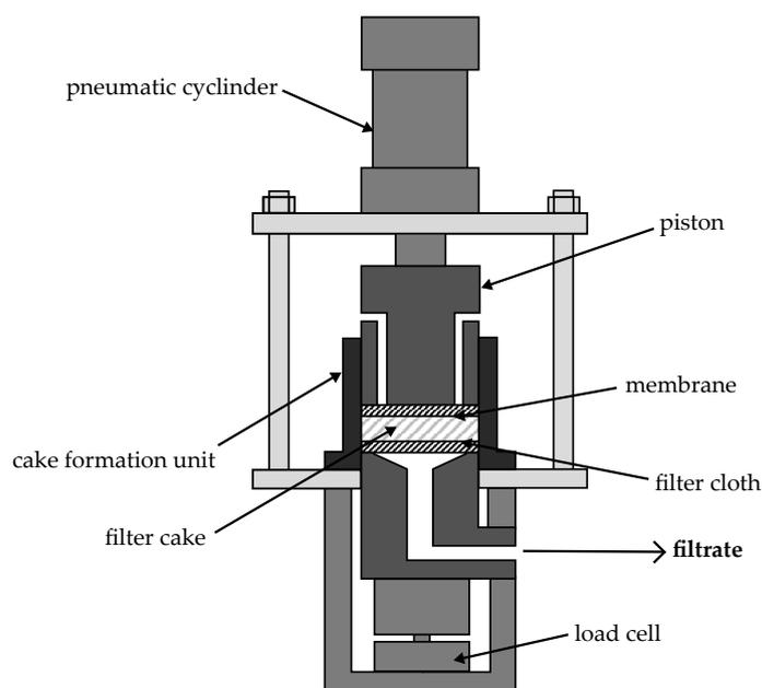
**Figure 3.** Setup of the compression–permeability cell developed by Alles [37]. The figure was taken from Yildiz et al. [33], reprinted with the permission of the publisher (Taylor & Francis Ltd., <http://www.tandfonline.com>, accessed on 23 January 2024).
