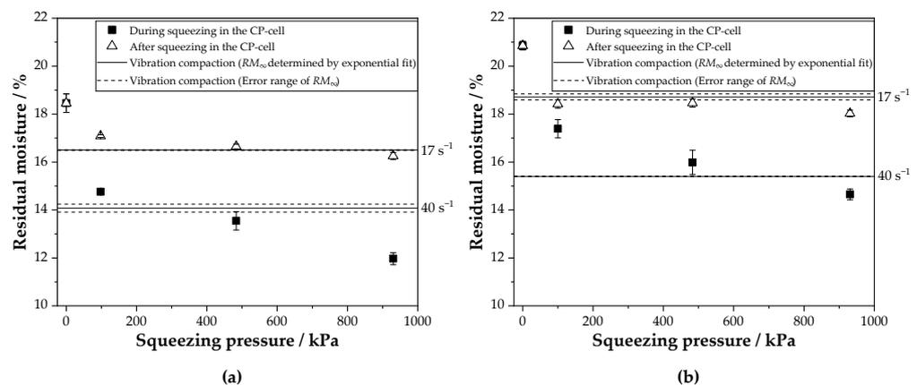
**Figure 8.** Minimum residual moisture of (a) homogeneous and (b) segregated filter cakes during and after squeezing at different pressures in the CP-cell and after vibration compaction. The values at a squeezing pressure of 0 kPa are the reference cake conditions after cake formation.
