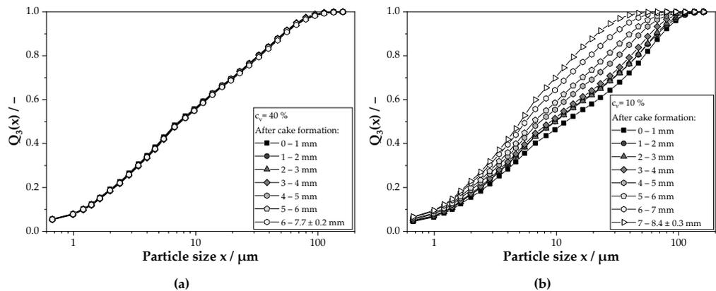
**Figure 5.** Cumulative particle size distribution in the different layers of a filter cake formed on a filter plate of a vibration apparatus from a slurry with a solid volume fraction of (a) 40% and (b) 10%. As the coordinate describing the filter cake height starts from the filter medium, the 0–1 mm layer is the lowest cake layer directly on the filter medium.
