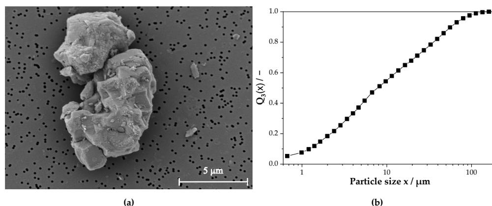
**Figure 1.** (a) Scanning electron microscope image of the model particles and (b) cumulative particle size distribution of the model material measured in deionized water with HELOS H0309 laser diffraction instrument (Sympatec GmbH, Germany).
