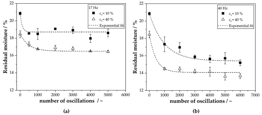
**Figure 6.** Residual moisture of homogeneous and segregated formed filter cakes after cake formation and vibration compaction at a frequency of (a) 17 Hz and (b) 40 Hz. The dashed line indicates the approximation of the data using Equation (6).
