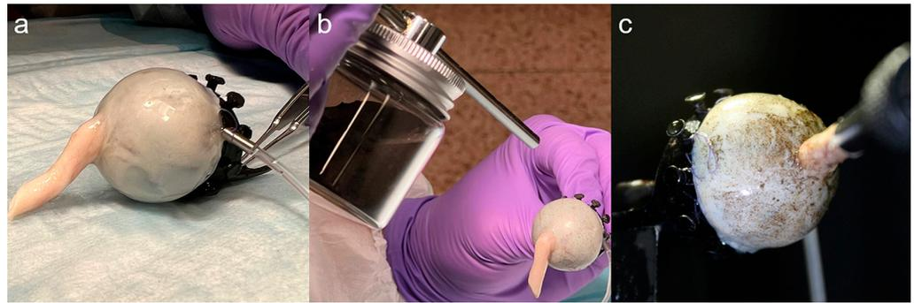
**Figure 2.** Sample preparation. (a) Globe was sutured to fixation ring, and infusion cannula inserted in anterior sclera over the pars plana. (b) Speckles of cast iron dust were randomly applied to the surface by using a pneumatic applicator. (c) Speckle pattern on the sclera permitted optical tracking of local scleral deformation.
